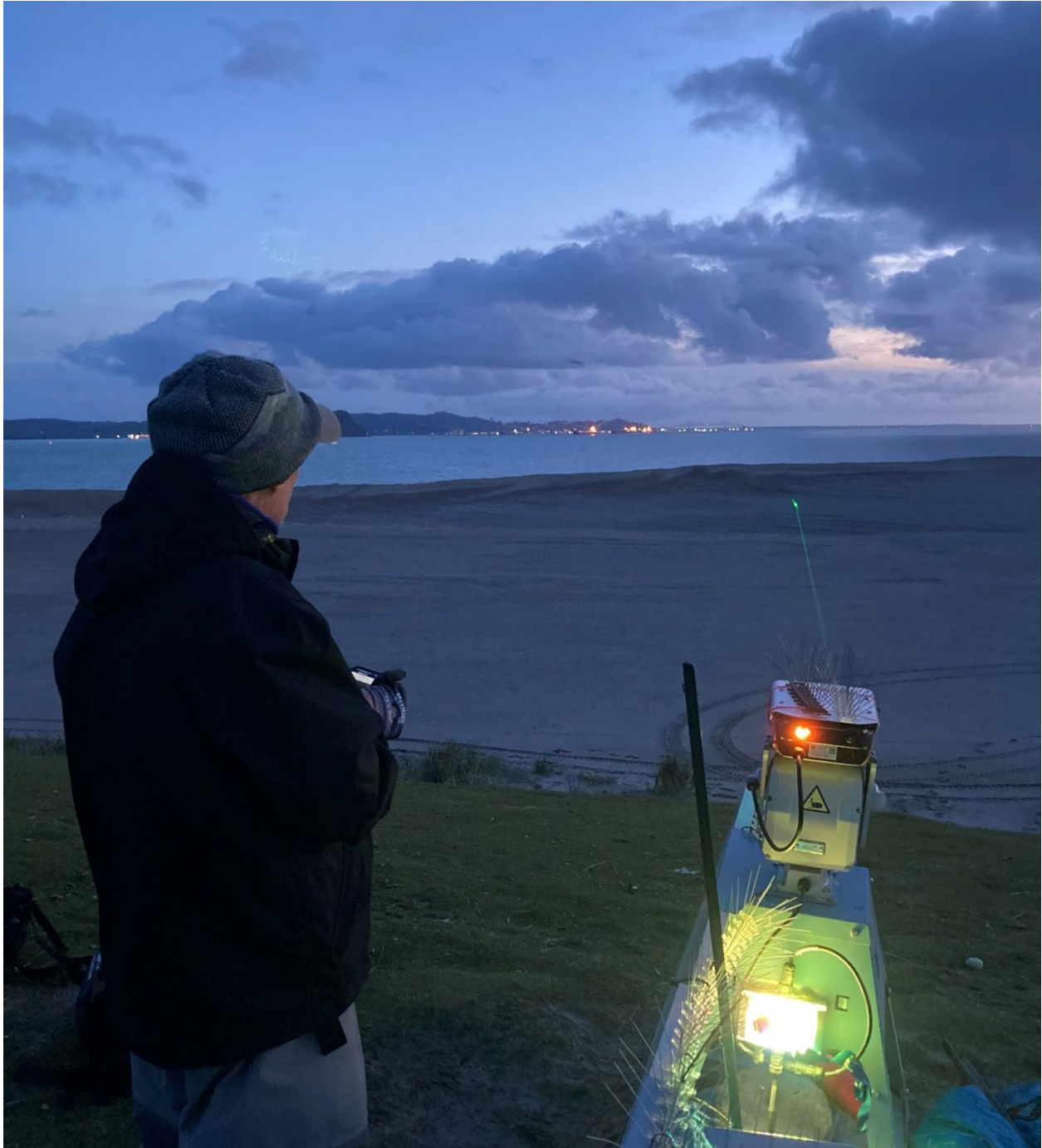
Figure 3. USACE Biologist observing the Avix Mark II Autonomous Laser® in operation. The sand berm around the 15.4-acre zone of coverage prevents overshooting by the beam. Photography by Erin Blair.
